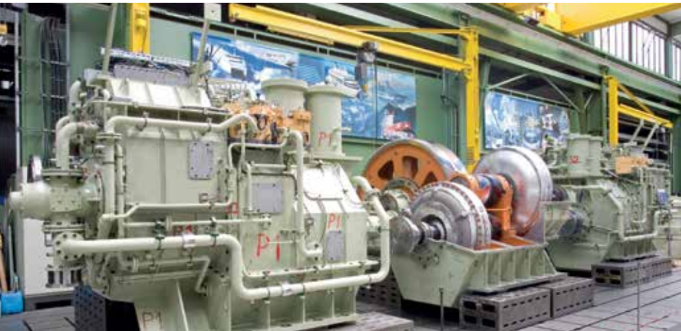
CODAD Gear with fluid couplings for 16 MW shaftline power
